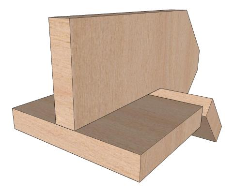
Drill and screw the shoe board to the frame.
