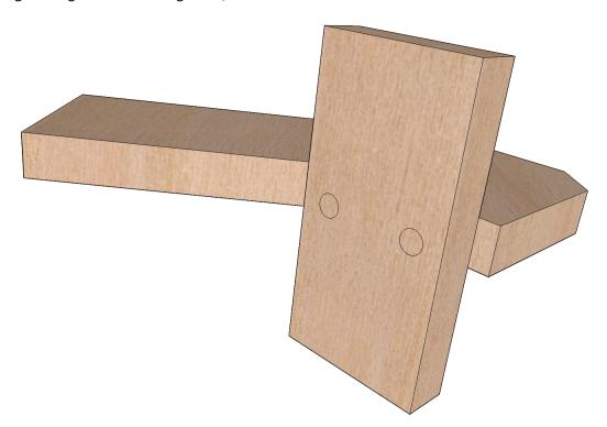
Drill and screw the sanding block to the frame.
