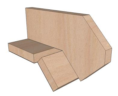
This is a sanding jig for sanding a 45 degree chamfer.
